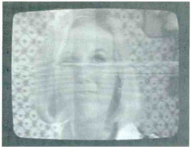
Fig. 1 Excessive input signals to a broadband amplifier often result in a faint negative picture from another channel appearing with the desired picture. When the horizontal blanking and sync pulses move sideways, the effect is called "windshield wiper".
