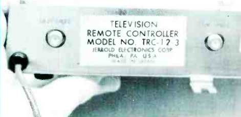
Fig. 2 Shielded "F" connectors are provided on the rear panel of the converter for the 75-ohm antenna wiring.
